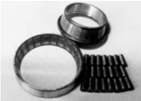
Fig. 15-12 Corrosion on Tapered Roller Bearing
